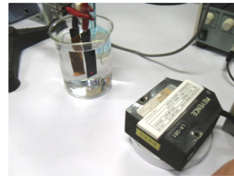
Fig. 4 Experimental scheme of electrochemical actuator in electrolyte solution using laser displacement sensor.
