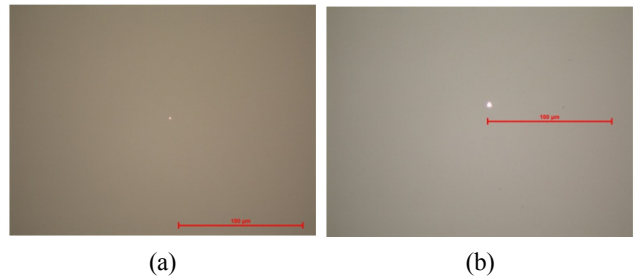
FIG. 9. Microscopic photographs of Al test defects with the diameter of (a) 3.0 \mu m, (b) 0.5 \mu m on the photo-mask.
