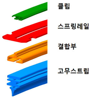
Fig. 2 Components consisting of a flat type blade
