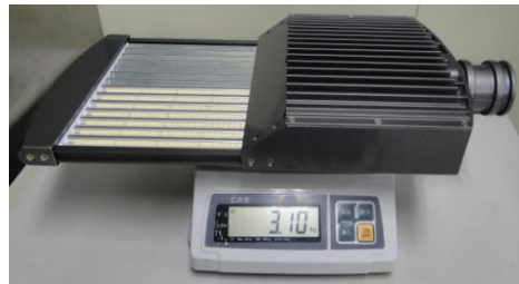
Fig. 15 Developed street-lighting system with the weight of 3.1 kg
