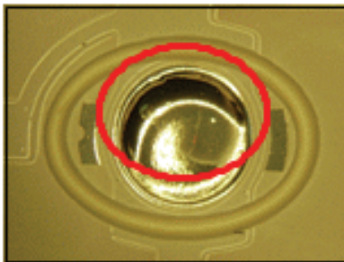
(c) Good plating of installed spot for LED chip Fig. 7 Good plating result by modified plating system
