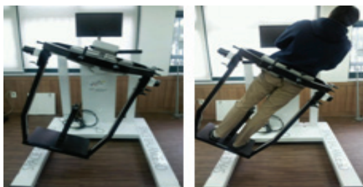
Fig. 1 Driving type of 3-D dynamic postural system (left; passive type, right; active type)
