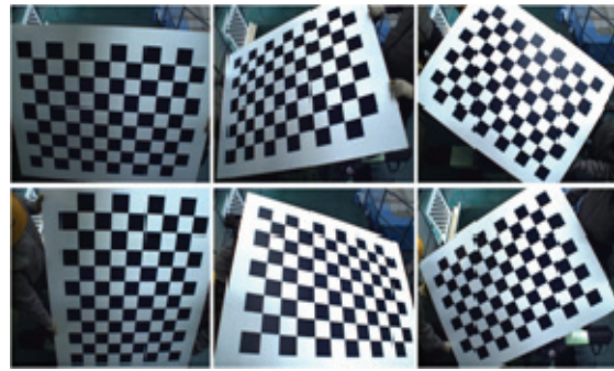
Fig. 6 Camera calibration with the calibration panel
