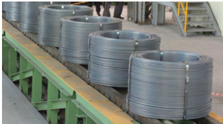
Fig. 1 Reinforcing bar in coils
