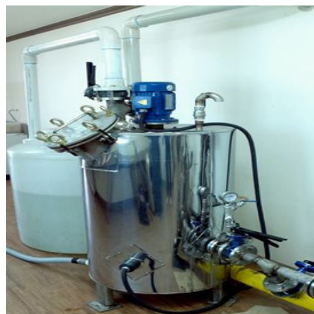
Fig. 1. Agitated storage tank (Left), TAO system (Right) for use in research.
