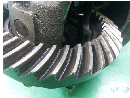
Fig. 7. Wear example of differential ring gear.
