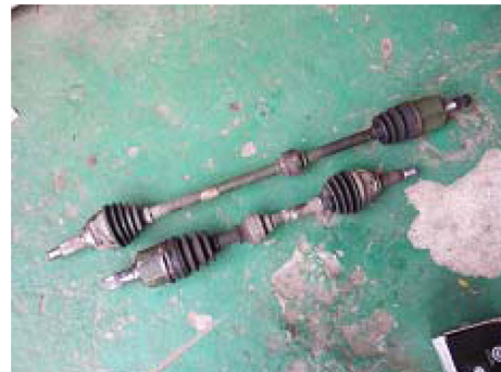
Fig. 4. Deformation example of constant velocity joint.
