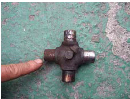
Fig. 5. Cross-section shaft wear example of propeller shaft.
