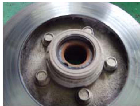
Fig. 6. Hub-bearing example stuck by leakage lubrication.
