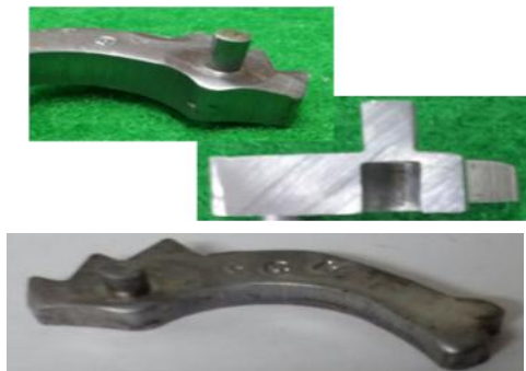
Fig. 16 The lock plate manufactured by the improved strip layout
