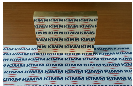
Fig. 6 Mirror surface obtained by ultra-fine planing using the developed hybrid machining system
