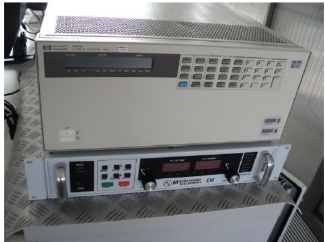
Fig. 3. Front panels of the fuel cell emulator Magna Power Electronics and the programmable electronic load HP 6050A.
