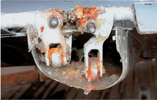
Fig. 3 Anti-icing fluid residue in elevator control stuck
