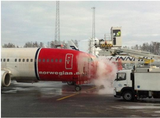
Fig. 1 Aircraft Ground De/Anti Icing in progress
