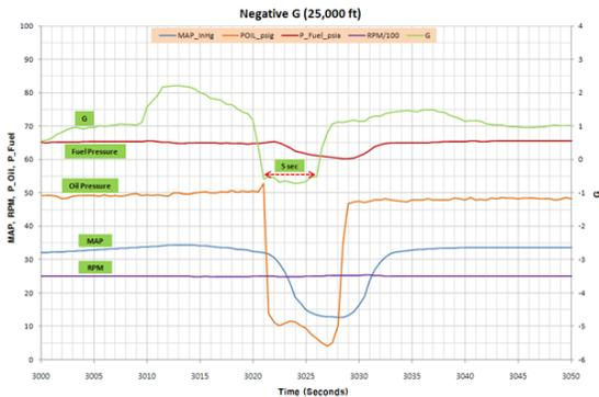
Fig. 7 Negative Acceleration Test(25kft)
