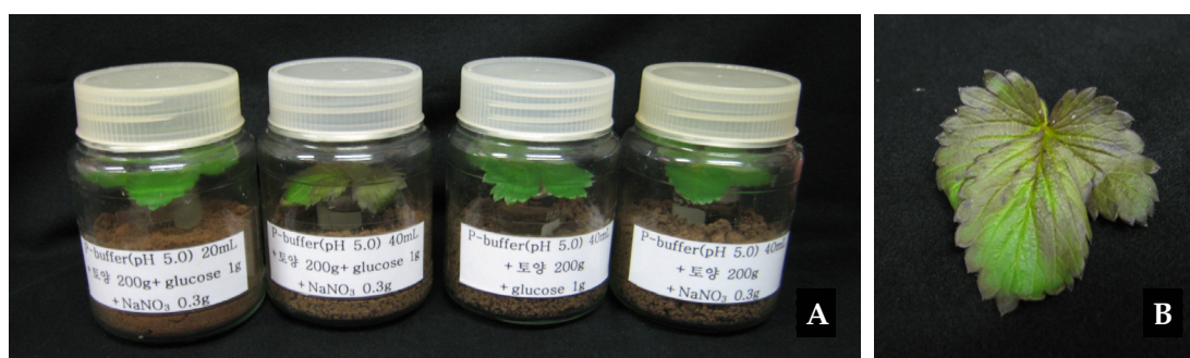
Fig. 1. Photograph showing the effect of various soil treatments on the damage to strawberry leaf caused by NO 2 gas produced from the soil during denitrification. A: (from left to right) Treatment 1, 2, 3, and 4. B: Strawberry leaf damaged by NO 2 gas produced from the soil in treatment 2. For the details of each treatment, see Table 2 in Materials and Methods section.
