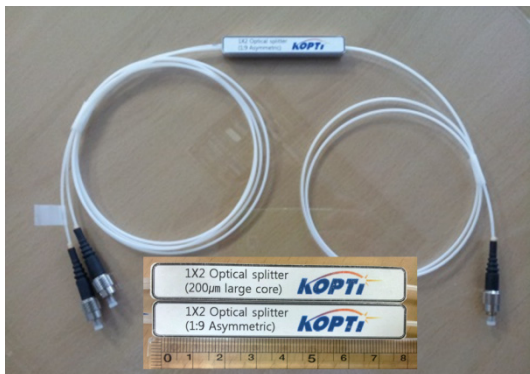
FIG. 10. Fabricated symmetric and asymmetric optical splitter.
