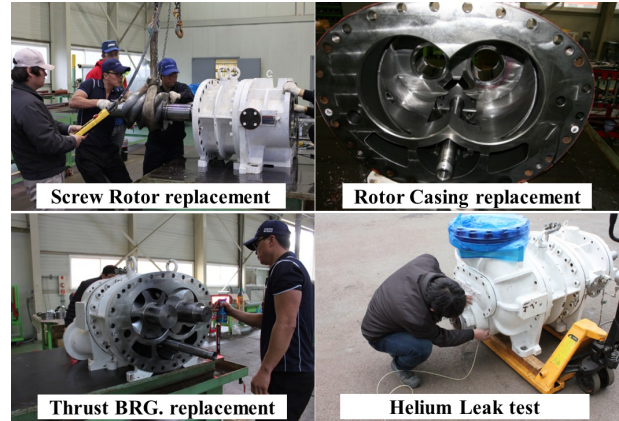
Fig. 3. Maintenance procedure of the compressor..
