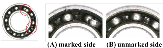
Fig. 4. Visual inspection of CC bearing interior.
