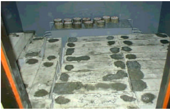
Fig. 2 RC specimens in accelerated chamber
