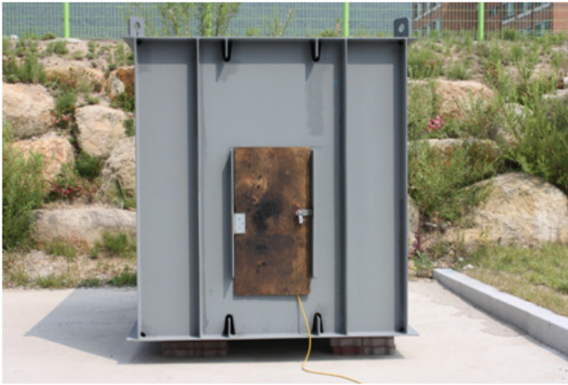
Fig. 5 Model Steel Box Girder Girder front photo
