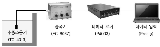
Fig. 3. Schematic diagram of equipment composition for measurement.
