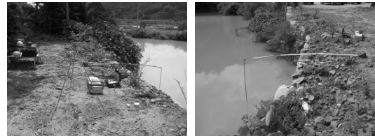
Fig. 8. Measurement of underwater noise and ground vibration (reservoir).
