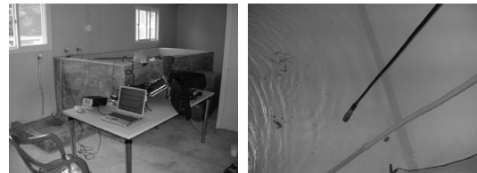
Fig. 9. Measurement of underwater noise and ground vibration (concrete water tank).
