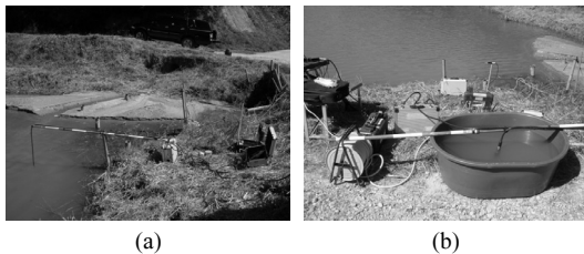
Fig. 5. Ground vibration and underwater noise measurement from reservoir(a) and water tank(b).
