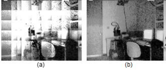
Fig. 6. Overlapping local regions; result of sum (a) and linear weighted blending (b)
