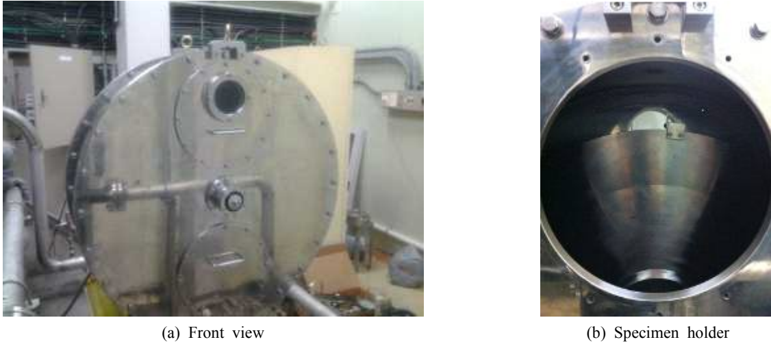
Fig. 1. Erosion-corrosion damage simulation apparatus.
