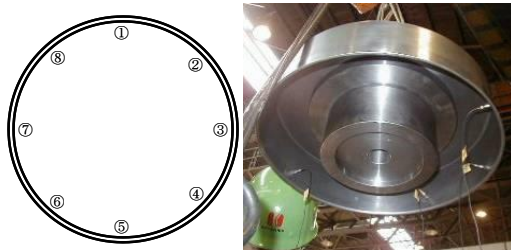
Fig. 9. Vibration measuring on the resonator
