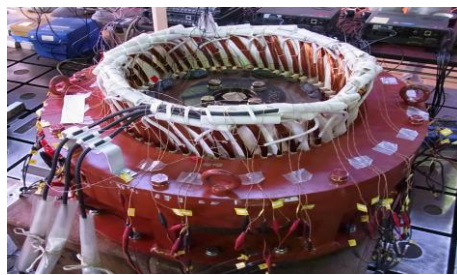
Fig. 10. Verification model with vibration measurement test
