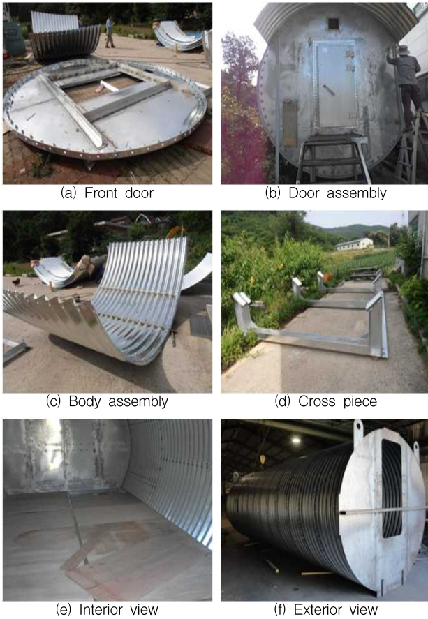
Figure 3. Manufacturing the cast-in-place structures using corrugated metal-plates
