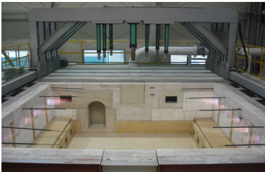
Figure 2. Fire test of high strength concrete
