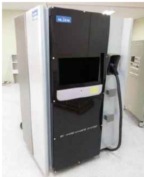
Fig. 12 Rapid EV charger proto-type
