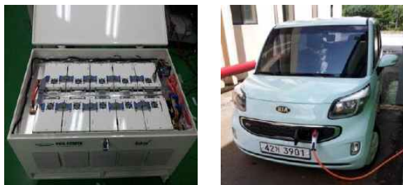
Fig. 14 Li-Ion polymer battery pack and electric vehicle used for testing the charger setup
