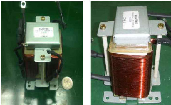
Fig. 4 Photo of coupled inductor used in the proto-type
