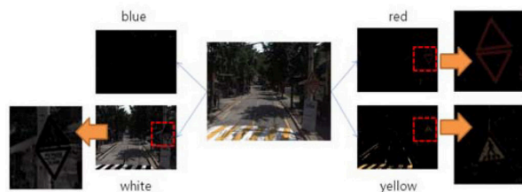
Fig. 2 Color Extraction Using HSV Color Space (E&G, 2012)
