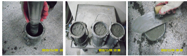
(a) Marshall compaction 15ea/layer (3 layers) (b) Vibration table 30sec/layer (3 layers) (c) Surface finish
