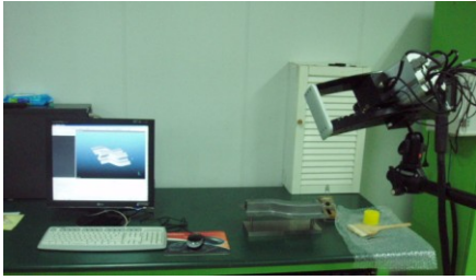
Fig. 7 Measurement of the 3-dimensional shape of the S-rail with a 3D optical scanner
