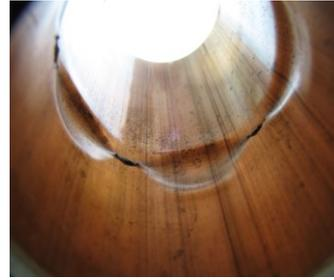
Fig. 2 Internal wrinkles around holes of hydroformed inner tube
