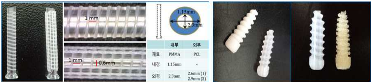
Fig. 5 Tube scaffold for tear duct (left), Screw scaffold for bone tissue engineering (right)
