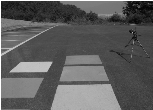
Fig. 10. Test construction, and thermal emission tester
