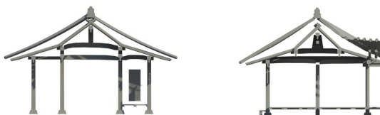
Fig. 13 Structural section combinations of the first bended-joint component of the inner residence
