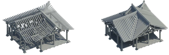
Fig. 14 Wooden structure and roof pattern of the first bended-joint component of the inner residence
