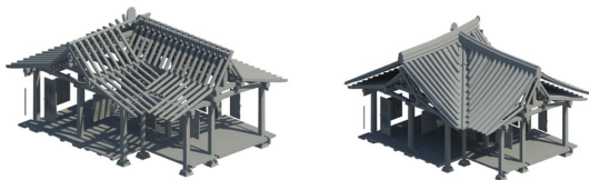
Fig. 16 Wooden structure and roof pattern of the second bended joint of the inner residence
