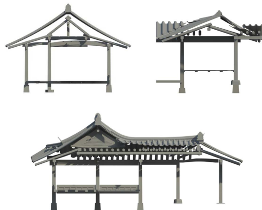
Fig. 9 Structure section combinations of the first bended joint components of the outer residence
