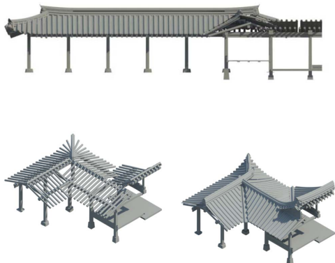
Fig. 10 The second Bended joint component of the Sarang-chaе and Daemun-chaе
