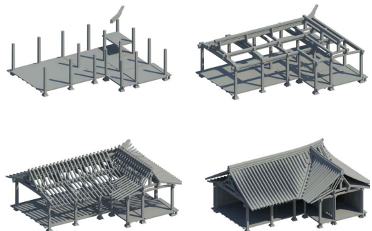
Fig. 7 Composition of base platform, body and roof parts
