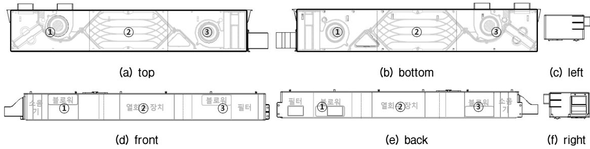
Fig. 8. Measurement positions of machine part.
