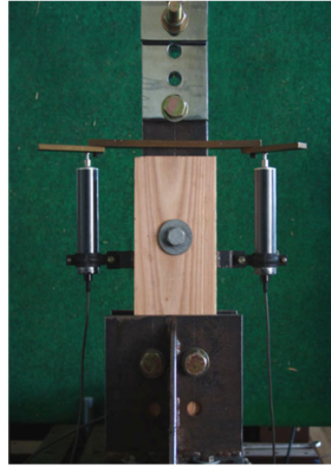
Fig. 2. Test of bolted joint with inserted steel plate parallel to the grain loading.
