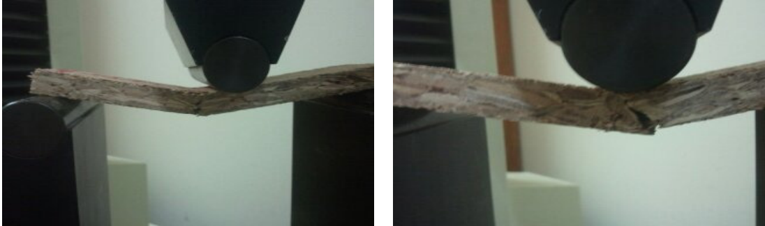
Fig. 2. Irregular site of crack on bending strength.
