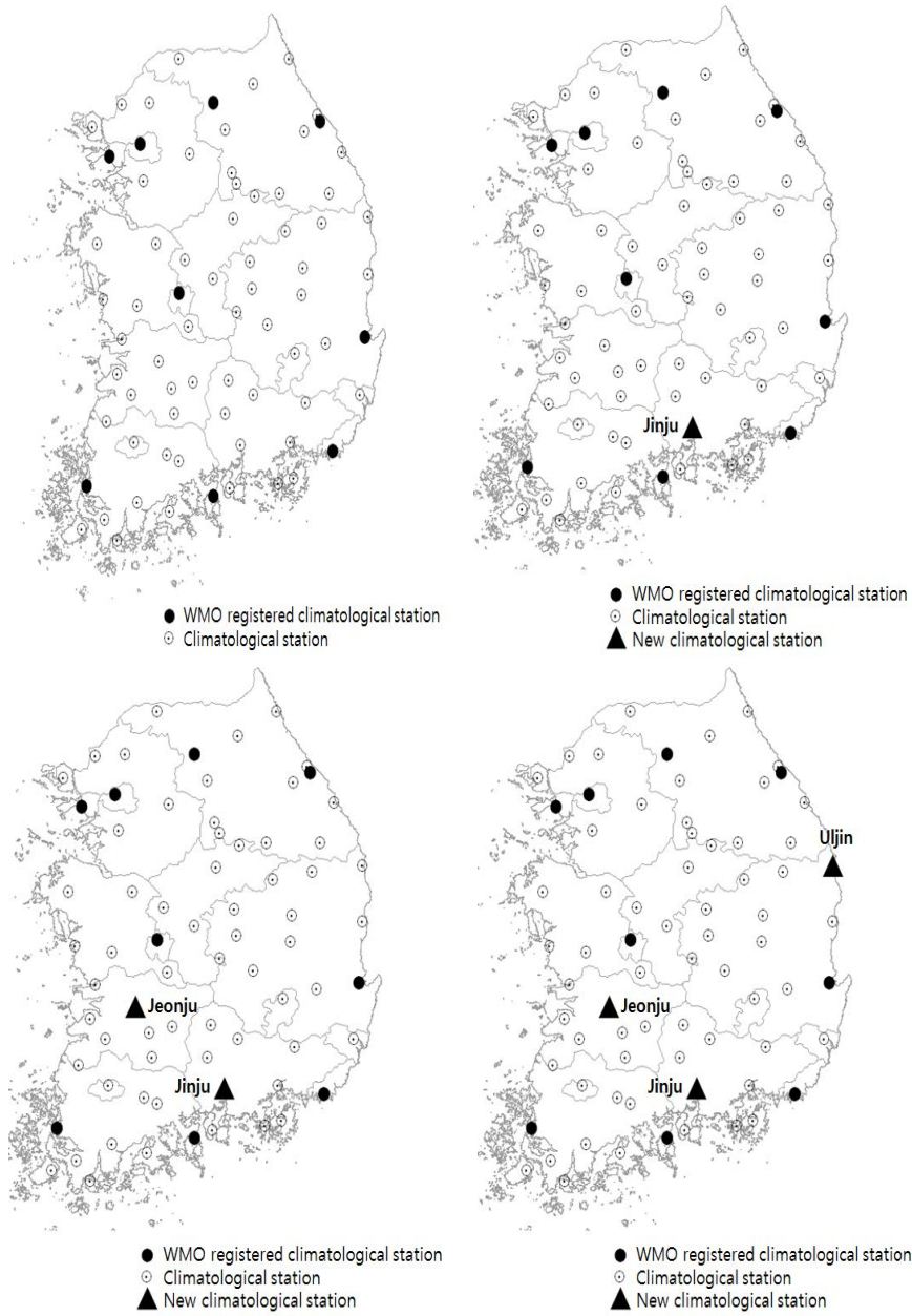
Figure 3.1 Sequential selection for new climatological stations by fractal dimension estimation (left upper; the existing climatological stations, right upper; first selection, left lower; second selection, right lower; third selection)
