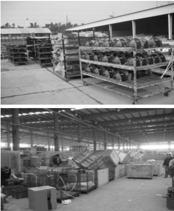
[Figure 3] Unpacking takes place in the buffer (top) and External storage area due to lack of space(bottom)
