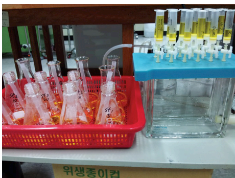
Fig. 3. Adsorption procedure in SPE.
