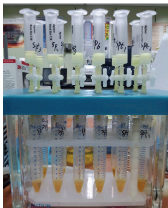
Fig. 4. Extraction procedure in SPE.
