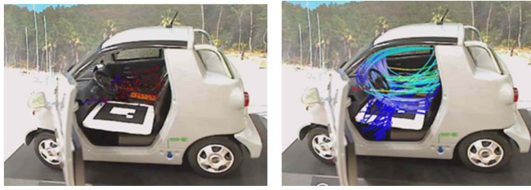
Fig. 16 AR-based air flow simulation inside a car
