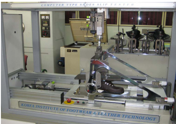
Figure 2. Shoe coefficient of friction measurement equipment
