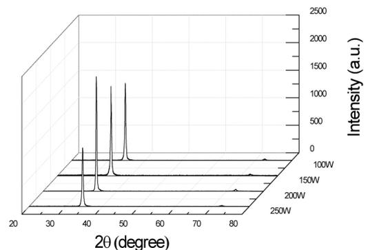
**Fig. 2.** XRD patterns of IGZO thin films prepared at RF powers ( $T_s = 300^\circ\text{C}$ ,  $P_w = 1 \text{ mTorr}$ ).
