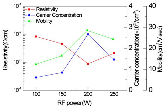
**Fig. 5.** Variations of resistivity, carrier concentration and carrier mobility of IGZO thin films with RF powers ( $T_S = 300^\circ\text{C}$ ,  $P_W = 1$  mTorr).
