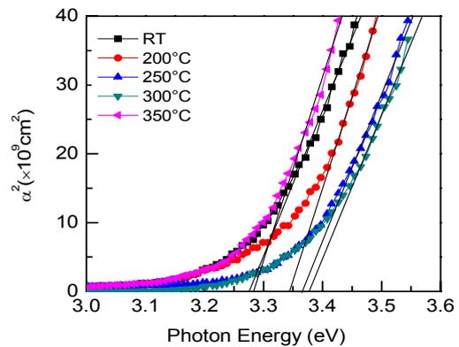
Fig. 13. Dependence of the optical band gap of IGZO thin films at different substrate temperatures ( $P_W = 1\text{ mTorr}$ ,  $P_{\text{RF}} = 200\text{ W}$ ).
