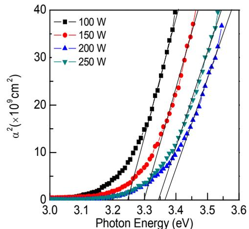
Fig. 9. Dependence of the optical band gap of IGZO thin films at different RF powers ( $T_s = 300^\circ\text{C}$ ,  $P_W = 1$  mTorr).
