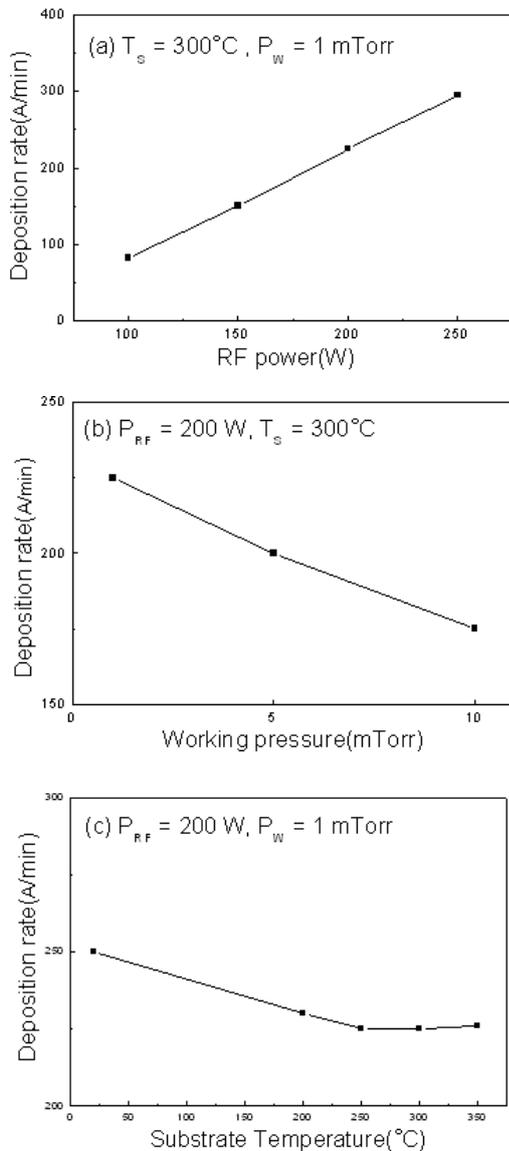
**Fig. 1.** Deposition rate of IGZO thin films as a function of (a) RF power, (b) working pressure, and (c) substrate temperature.
