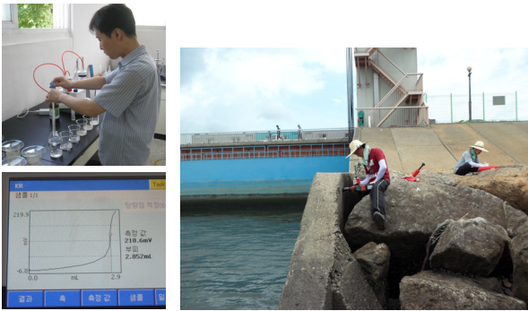
(a) Titration (b) At Field Photo 1 Chloride contents analysis and field test
