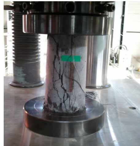
Fig. 2 Compressive strength test setup
