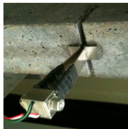
Fig. 1 Test method and test setup for notched beams
