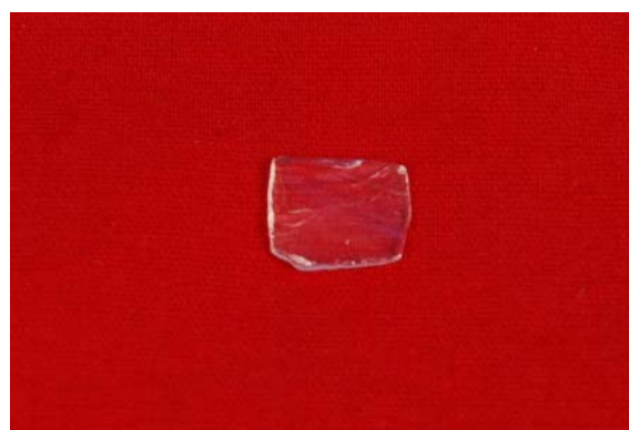
Figure 1. Photograph of as-grown LASO crystal.
