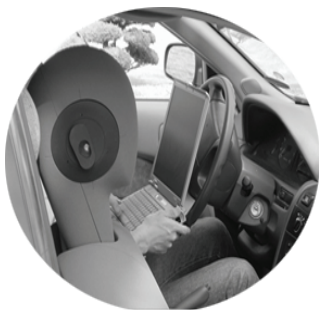
Fig. 5 Pictorial illustration of a binaural acoustic head for recording interior sound inside a passenger car
