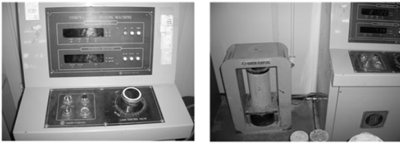
Fig. 7 Concrete compressive strength test.
