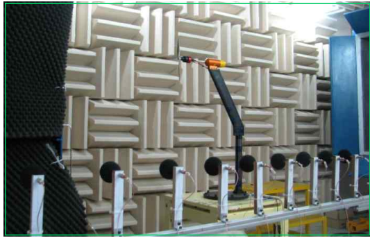
Fig. 2. Wind tunnel test jig for noise test
