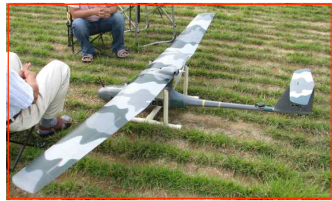
Fig. 4. Fixed wing UAV for noise test [Remo Eye 006, UCON system]
