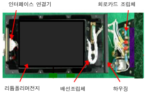
Fig. 6. Electric power supply
